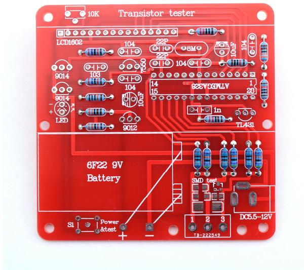
The electrode of the electrolytic capacitor should be aligned with the PCB side with white line.
