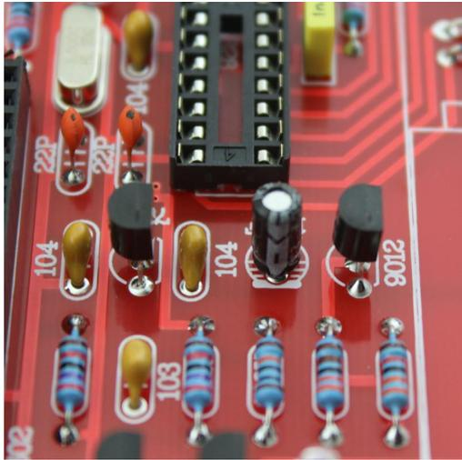
After all the welding jobs have been done, please connect the electric power instead of connecting Atmega328 and LCD(9V battery or external 5.5-12V DC power, outside -, inside +), and measuring the voltage of the pin7 and pin22 on the IC plug by using the multi-meter, and the voltage should be +5V(the button should be pushed when measuring), which means the circuit and power are working in normal condition.
