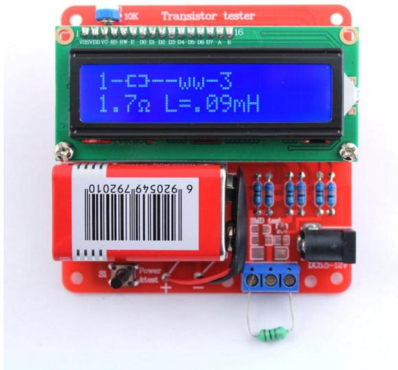
For resistors below  $2100\Omega$  also the measurement of inductance will be done. The range will be from about  $0.01\text{mH}$  to more than  $20\text{H}$ , but the accuracy is not good. The measurement result is only shown with a single component connected.
