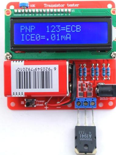
Display the Collector cutoff current  $I_{ce0}$  with currentless base (10uA units) and Collector residual current  $I_{ces}$  with base hold to emitter level . This values are only shown, if they are not zero (especially for Germanium transistors).
