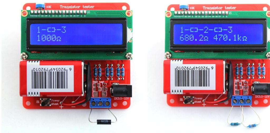
Up to two Resistors are measured and shown with symbols and values with up to four decimal digits in the right dimension. All symbols are surrounded by the probe numbers of the Tester (1-3). So Potentiometer can also be measured. If the Potentiometer is adjusted to one of its ends, the Tester cannot differ the middle pin and the end pin. Resolution of resistor measurement is now up to 0.01Ω, values up to 50MΩ are detected.
