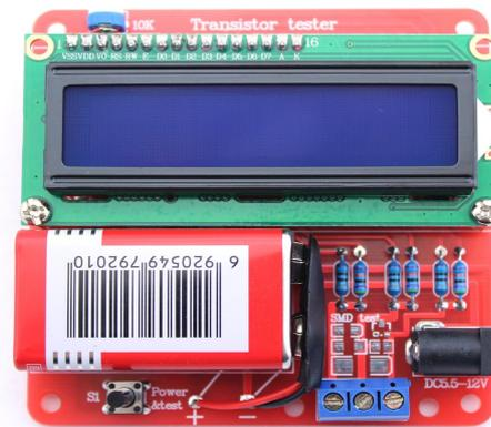
After all the installation, connect the power. Push the button, and maybe the screen will light without any character display. Don't be panic, right adjust the resistance and you will see the character.
